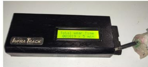
Fig. 2. Wear time after 1 week (1019x5 minutes = 5095 minutes, i.e., 84.91 hours total, or 12.1 h/d on average).
